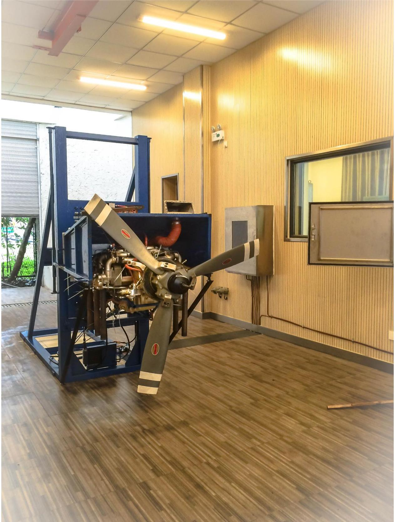
*Picture 3: Overhauled io-360-ES on test on mobile test bench*
